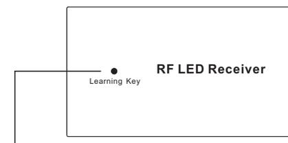
**Step 2:** Click the "Learning Key" button on RF receiver or re-power on the receiver three times continuously to set it into pairing status
